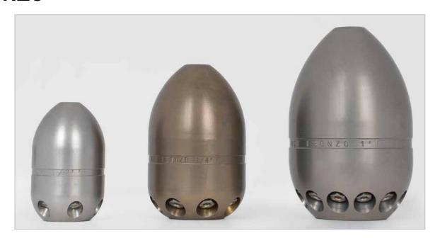
Grenade nozzles made of hardened stainless steel, for cleaning operation in concrete pipes. **Ceramic inserts** are set as standard configuration, **carbide inserts** (for water recycling units) upon request.
