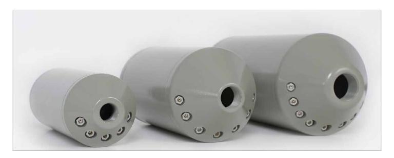
**Self-balancing heavy nozzles**, torpedo shaped, for bottom cleaning and sand removal applications. These nozzles are designed and manufactured so that the water is always oriented to the bottom of the pipe, just for sediments removal (and not for all around cleaning), **optimizing water consumption**. **Ceramic inserts** are set as standard configuration, **carbide inserts** (for water recycling units) upon request.
